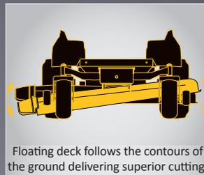
Floating deck follows the contours of the ground delivering superior cutting.
