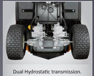
Dual Hydrostatic transmission.
