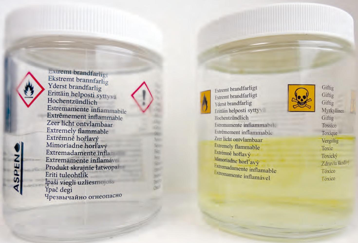
Aspen fuel on the left compared with regular pump fuel on the right
