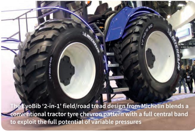
The EvoBib '2-in-1' field/road tread design from Michelin blends a conventional tractor tyre chevron pattern with a full central band to exploit the full potential of variable pressures
