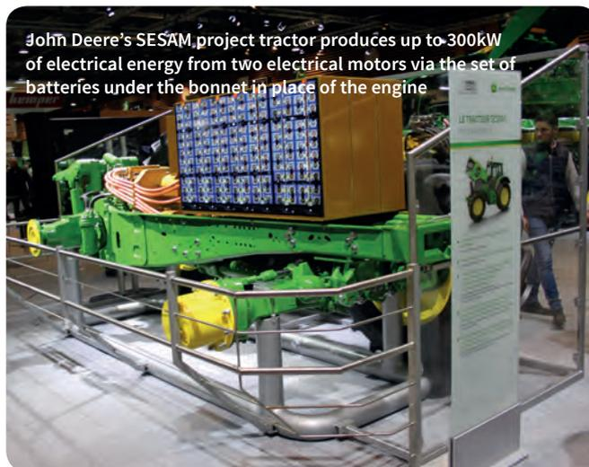
John Deere's SESAM project tractor produces up to 300kW of electrical energy from two electrical motors via the set of batteries under the bonnet in place of the engine.
