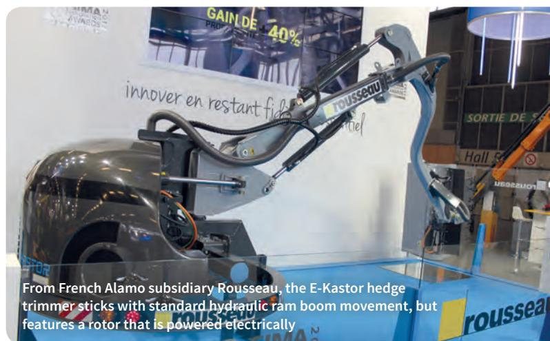
From French Alamo subsidiary Rousseau, the E-Kastor hedge trimmer sticks with standard hydraulic ram boom movement, but features a rotor that is powered electrically
