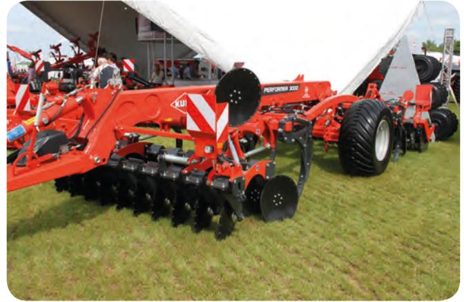
Cultivation and drilling equipment from bigger names included a 3m version of Kuhn's Performer deep-working disc/tine cultivator. Key components include two rows of 510mm independent and hydraulically adjustable discs and four rows of non-stop hydraulic breakback tines capable of working to a maximum depth of 350mm. Tine point choices include standard 80mm shares, 50mm subsoiling shares or wing shares. At the rear is a notched roller providing up to 225kg/m of hydraulically adjustable pressure.
