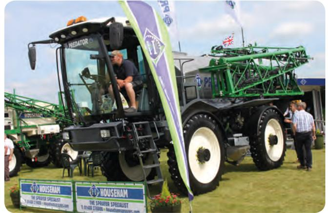
A new flagship self-propelled sprayer from Househam is the Predator, available in 4,000 and 5,000-litre capacities, with booms to 36m. Innovations on the machine include a hydraulic load-sensing suspension system which adapts responsiveness according to tank load. The engine is a four-cylinder MTU producing 230hp, and unladen weight is 10 tonnes.
