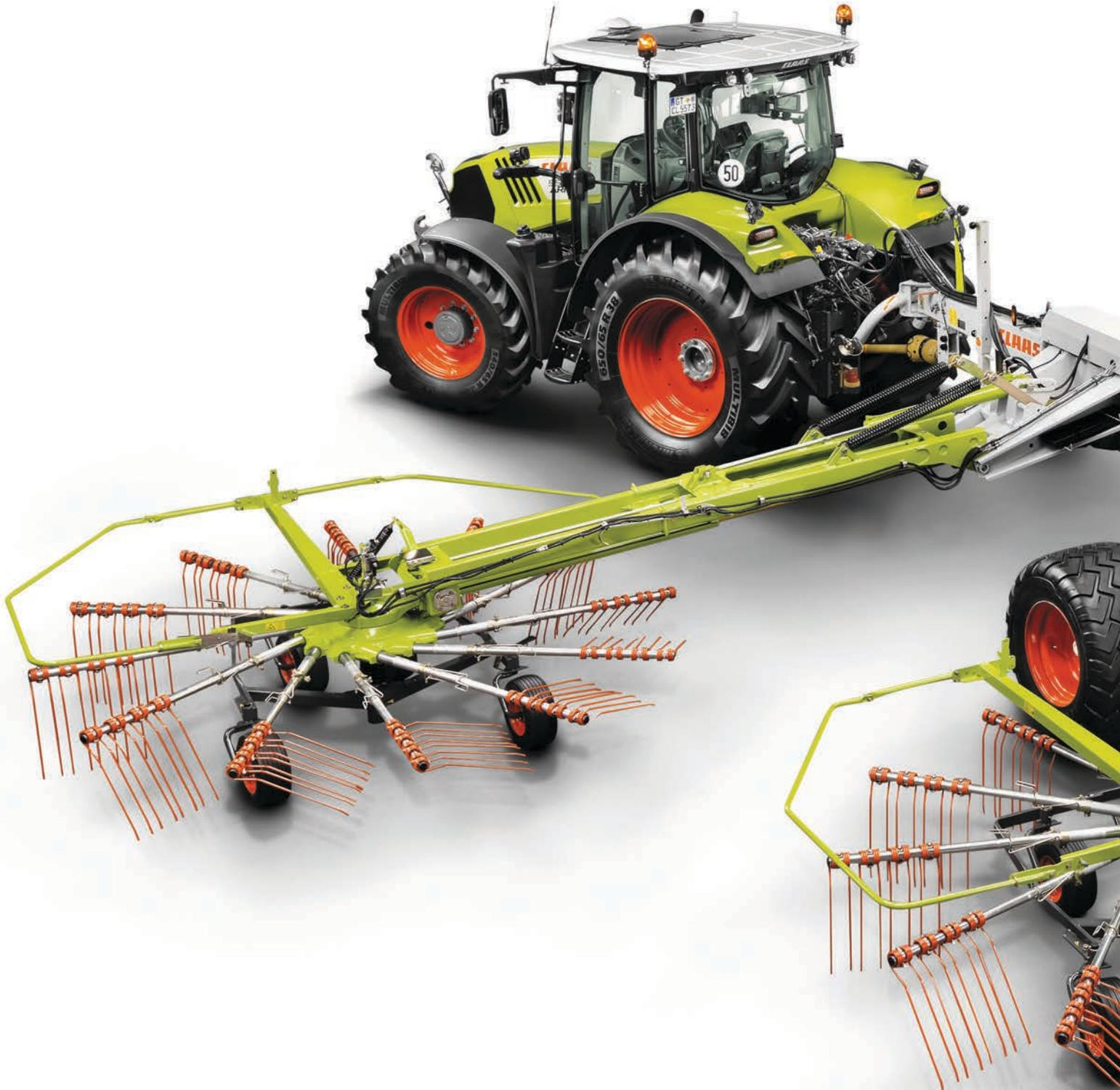
In order to achieve an even, consistent swath for high output foragers and balers, Claas has introduced a new rake, the Liner 3600, on which the working width can be adjusted from 9.90m up to 12.50m, but is designed so that it is compact to transport on the road.
