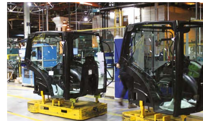
Cabs frames from the Croix plant in France are trimmed and finished at Basildon as part of tractor assembly
