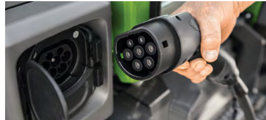
While AC charging is generally an overnight exercise, DC fast charging with up to 80kW charging power makes charging from 20% capacity to 80% possible in around 45 minutes
