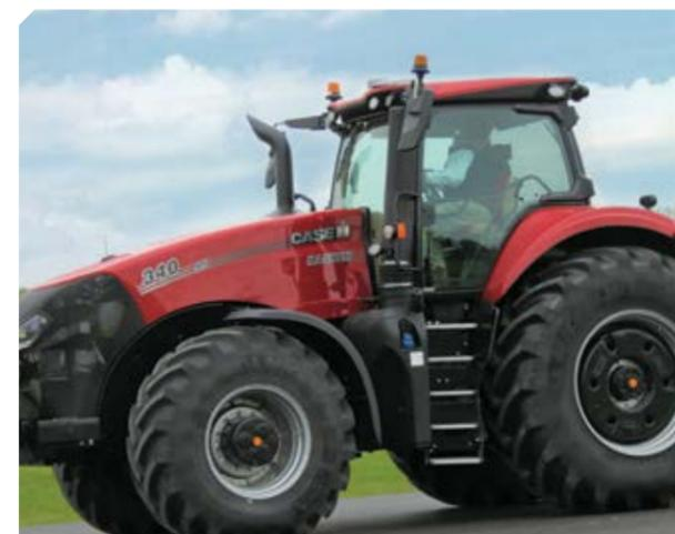
**External changes are relatively minor, but include a new nose styling, optional LED lighting and cameras, plus a full-length door with a remote locking/unlocking key fob**
