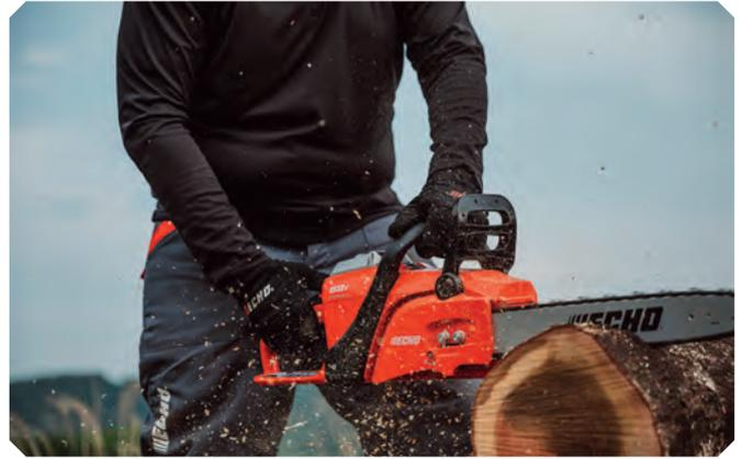
and the oil tank is translucent for easy level checks. The power comes from the brushless motor which Echo says requires minimal maintenance due to non-wearing parts.
