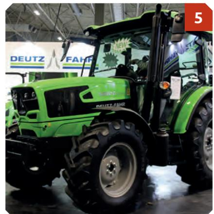
Maximum speed of 40km/h can be reached at 1,870 engine rpm on all models, and all are equipped as standard with four-wheel drive and four-wheel braking. Four-wheel drive operation and the differential lock can be electro-hydraulically operated as an option.
