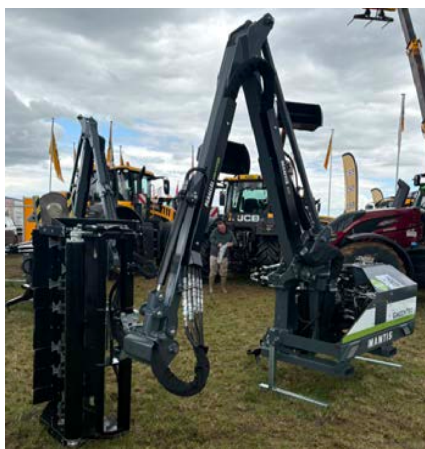
Based on Razorback technology, mounting of GreenTec's new Mantis 570S to the tractor is via a patented four-point design
