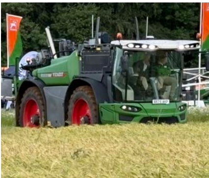
New 'Gen 2' versions of Fendt's 600 series Rogator sprayers feature improved OptiNozzle drift reduction automatic selection technology
