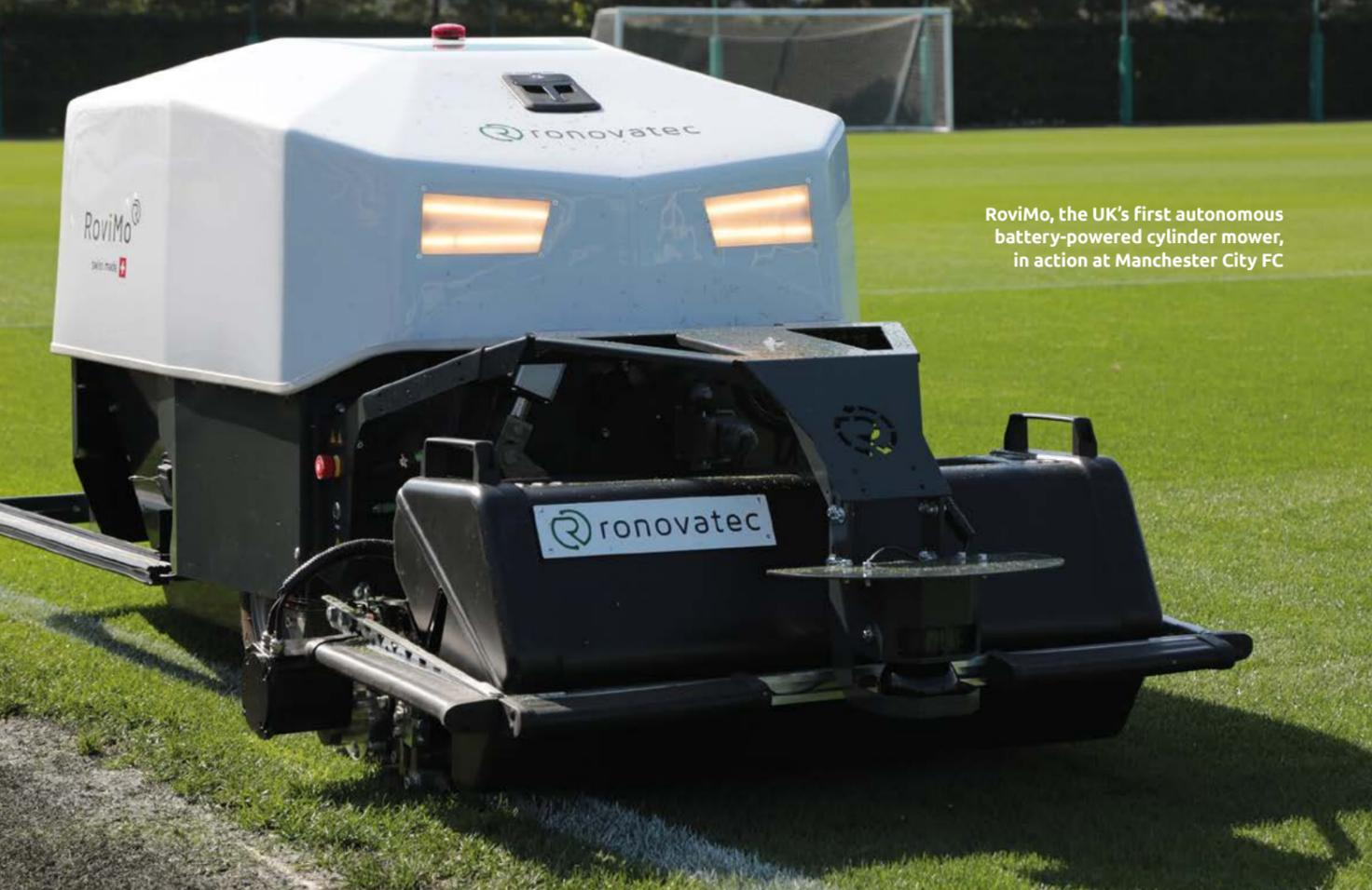
RoviMo, the UK's first autonomous battery-powered cylinder mower, in action at Manchester City FC
