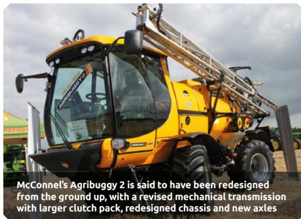
McConnell's Agribuggy 2 is said to have been redesigned from the ground up, with a revised mechanical transmission with larger clutch pack, redesigned chassis and new axles
