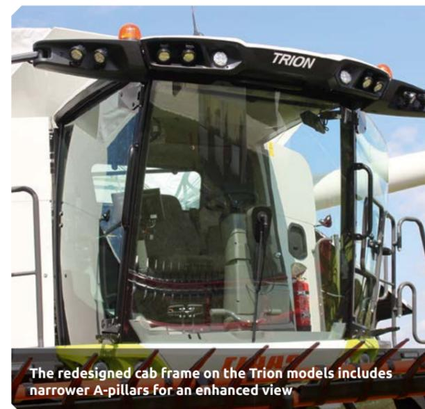
The redesigned cab frame on the Trion models includes narrower A-pillars for an enhanced view
