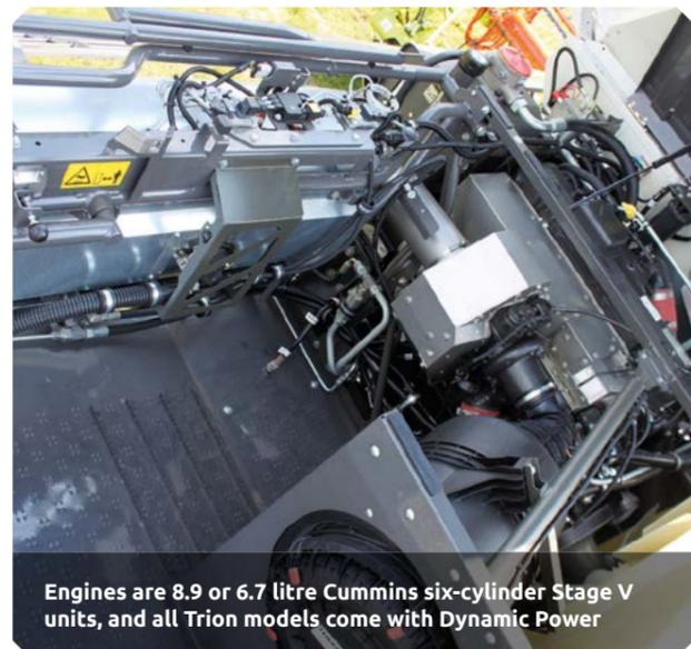
Engines are 8.9 or 6.7 litre Cummins six-cylinder Stage V units, and all Trion models come with Dynamic Power
