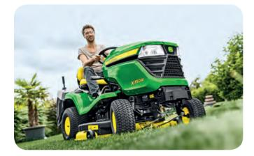
top to allow a clean flow of grass cuttings for a quality cut, even in normally difficult tall grass. The stamped steel design of the durable heavy-duty deck eliminates sharp edges and corners where material can build up and compromise performance. John Deere says the new Accel Deep deck ensures a premium finish, as well as many hours of trouble-free operation.
