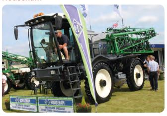
A new flagship self-propelled sprayer from Househam is the Predator, available in 4,000 and 5,000-litre capacities, with booms to 36m. Innovations on the machine include a hydraulic load-sensing suspension system which adapts responsiveness according to tank load. The engine is a four-cylinder MTU producing 230hp, and unladen weight is 10 tonnes.
