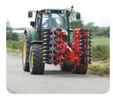
tractor when attached, ensuring that it follows the nose of the tractor, steering smoothly even at speed. The headstocks are designed to take the forces produced even when using a shattaboard.
