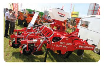
Simplicity was also a theme with the Split-Level subsoiler from Bristows, a firm based not far from the Cereals site. Targeted at the oilseed rape establishment market, it can be specified with leading loosening tines or discs, which precede subsoiler legs of various types depending on the level of shattering and surface movement required.
