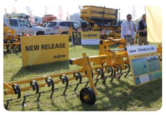
Making its debut on the Claydon stand was the firm's front linkage-mounted Terrablade inter-row hoe, designed for shallow working between wide-row band-sown crops established using one of the company's drills to reduce demands on herbicides and cut crop protection bills. Claydon says the Terrablade can be used at forward speeds of approximately 6.0km/hr, working at up to 20mm deep. Guide wheels are installed at the front of the implement.
