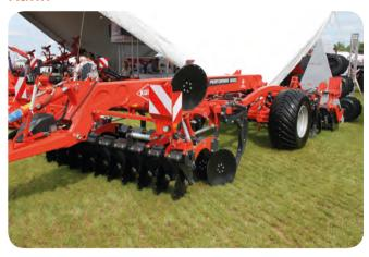
Cultivation and drilling equipment from bigger names included a 3m version of Kuhn's Performer deepworking disc/tine cultivator. Key components include two rows of 510mm independent and hydraulically adjustable discs and four rows of non-stop hydraulic breakback tines capable of working to a maximum depth of 350mm. Tine point choices include standard 80mm shares, 50mm subsoiling shares or wing shares. At the rear is a notched roller providing up to 225kg/m of hydraulically adjustable pressure.
