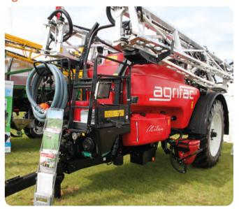
In the sprayer lines, a number of makers debuted new products. On sale in mainland Europe for a number of years, Dutch manufacturer Agrifac is now offering the trailed Milan range alongside its established Condor self-propelled sprayers, the two sharing similar plumbing. There are 3,500, 4,200, 5,400 and 6,800-litre tank options, with booms from 27-45m, and individual nozzle section control available.
