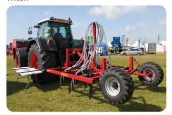
Farm designed and built, the Triton drill was attracting a lot of attention on the working plots, largely because of its simplicity, which is said to ensure it moves the minimum amount of soil to avoid disturbing weed seed, while still filling the seed slot.
