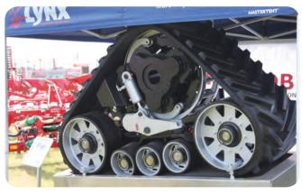
Retro-fit rear track units have found homes with a number of UK cropping businesses seeking increased traction and flotation from high-hp tractors yet wanting a fully wheeled tractor at other times of the year, but the downside for many is the 40% reduction in road speed that they impose. Lynx Engineering is now offering a new 40km/hr (25mph) rated system from Dutch maker Zuidberg.
