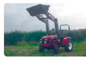
which is a self-levelling loader designed specifically for the 254CH. The loader offers a lift capacity of 400kg and a digging depth of 140mm. The bucket has a 0.2 m cu capacity.
