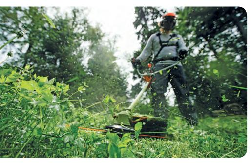
The range of High Torque brushcutters with a 1:2 gear reduction ratio, deliver up to 50% more torque at the cutting head compared with previous models. What this means is a High Torque brushcutter can provide the same cutting performance as a considerably larger machine but with a smaller, lighter engine.
