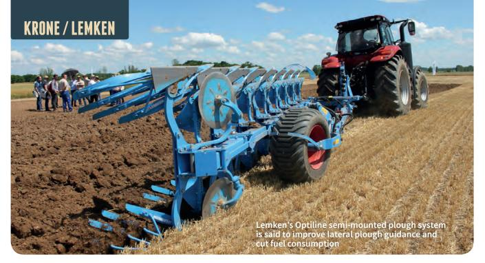
of up to 10%, while pointing out that ploughing without lateral pull cuts operator strain, eliminating the need to counter-steer. Operators are able to optimally adjust the plough's landside pressure and the tractor's lateral pull via Optiline's hydraulic adjustment, also aiding consistent front furrow widths.
