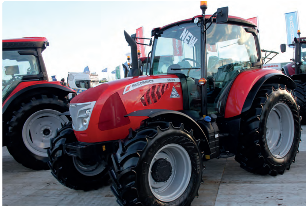
Three new X6 four-cylinder McCormick tractors span 110-126hp, combining X5 accommodation with the existing X6 transmission
