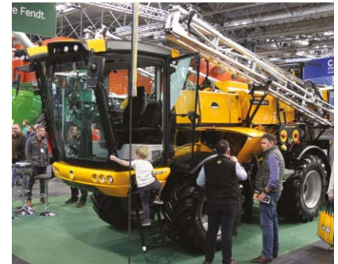
The latest McConnell Agribuggy features a hydro-mechanical transmission
