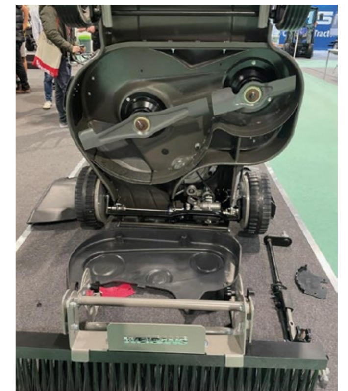
Weibang featured an offset twin-blade mulcher
