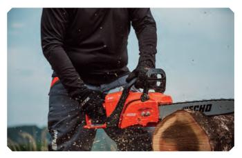
and the oil tank is translucent for easy level checks. The power comes from the brushless motor which Echo says requires minimal maintenance due to non-wearing parts.
