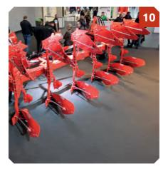
into the six-nine furrow class, the semi-mounted Mirco line **(\*pic 10)** has a simple remove pin/operate ram switching process when changing between on-land and infurrow work, and a 100-degree headstock pivot for tight headland turns.
