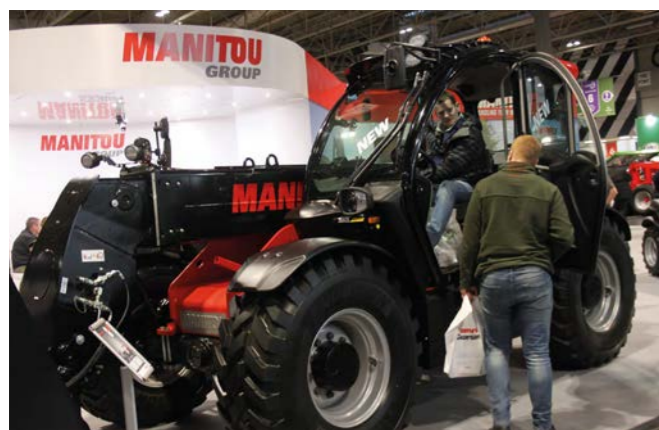
With maximum lift capacity/height figures of 5,000kg/7.6m, Manitou's MLT 850-145V+ slots in above the MLT 841 and beneath the 961 and 1041 in the NewAg XL range
