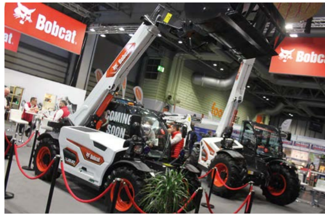
Bobcat's new TL25.60 'super compact' telehandler has a maximum lift capacity of 2,500kg, maximum lift height of 5.91m and maximum reach of 3.31m
