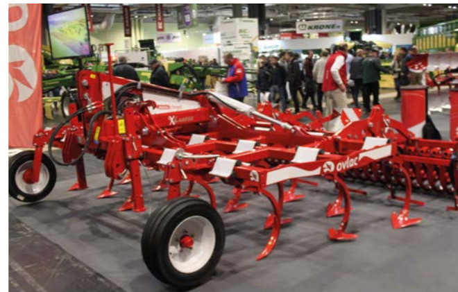
Ovlac, which is looking to fill some UK dealer network gaps, showed its Mini Chisel, a cultivator incorporating a claimed-unique rubber stone protection break-back
