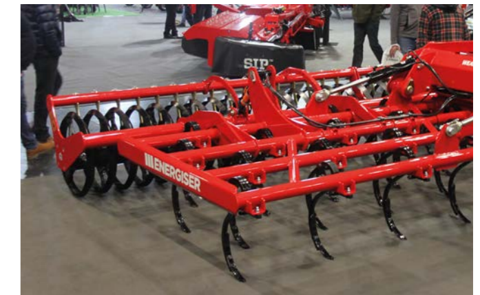
Weaving's Energiser is a 6m shallow cultivator for seedbed preparation, straw redistribution and soil loosening down to 150mm
