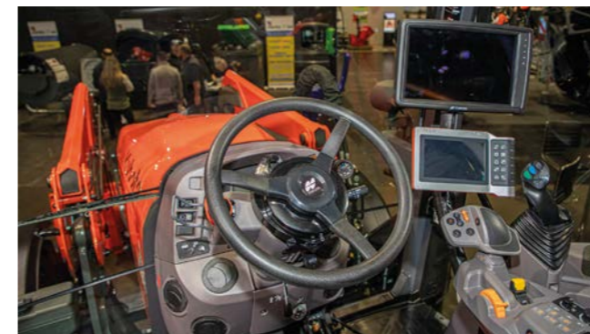
A new range of auto-steer options for Kubota's M-series tractors comes courtesy of a European-wide agreement with Topcon Positioning Systems
