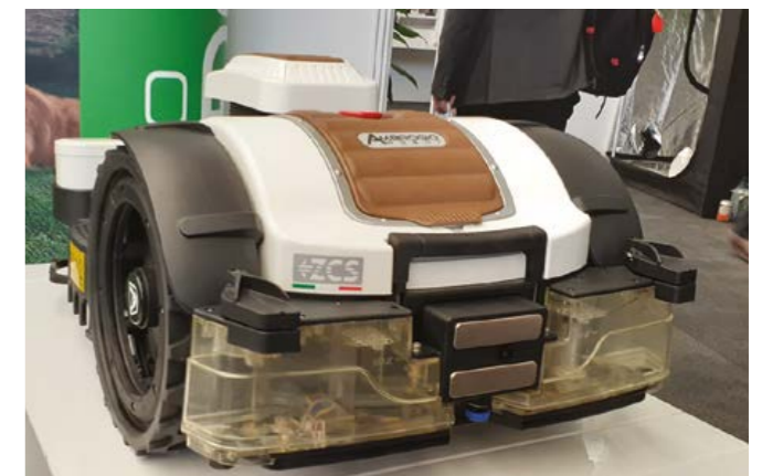
The Ambrogio robot, featuring the ZDefence sprayer attachment
