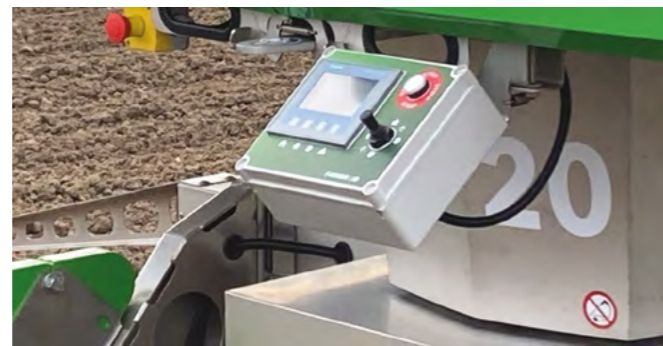
An on-board controller is used for initial machine placement within the field. RTK receivers front and rear work with an on-farm base station
