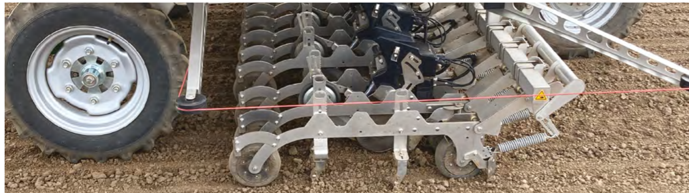
The machine uses a combination of weeding wires and blades to remove weeds between and within rows, based on records of each seed's sown location
