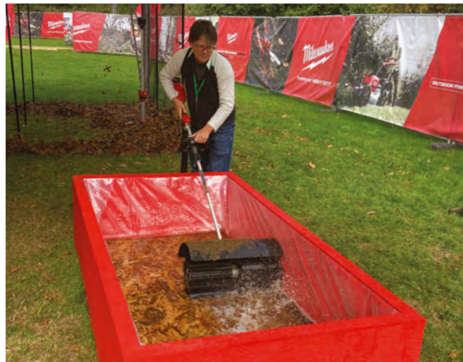
Quik-Lok interchangeable heads for the M18 18V attachment range includes rubber broom and bristle brush attachments to clean concrete of mud, slurry and leaves
