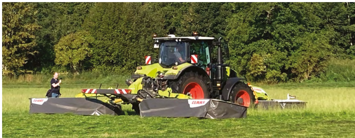
At 9.7-9.9m, the new Disco 1010 Trend is the widest mounted mower without a telescopic boom on the market, claims Claas
