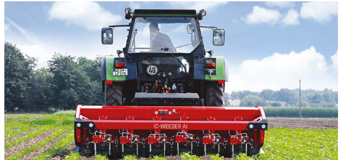
The Steketee automatic intra-row hoeing IC-Weeder uses artificial intelligence for guidance in removing weeds between sugar beet rows
