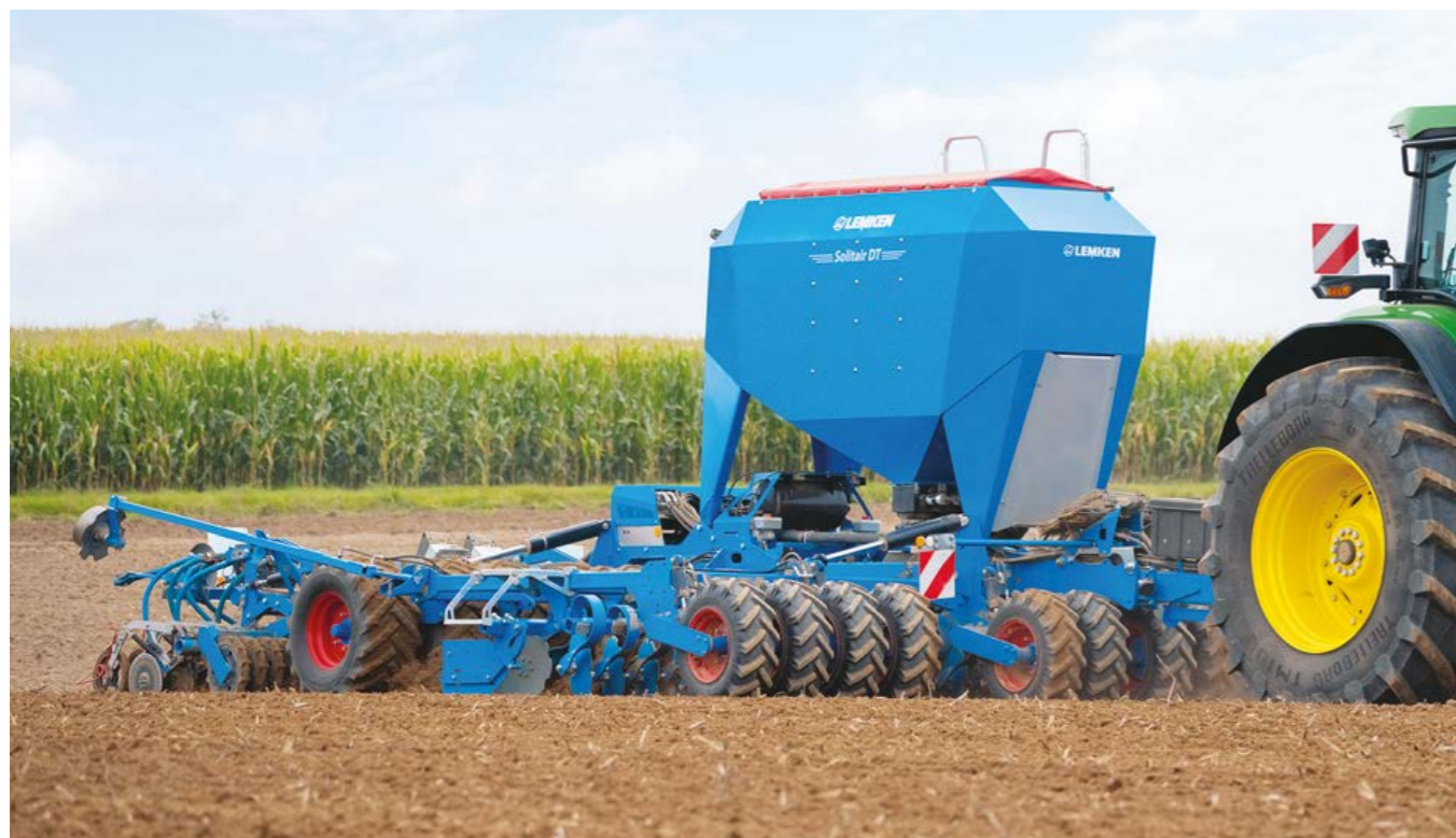
Lemken claims potential diesel consumption figures as low as 5.0 l/ha for the new low-draught design 4.0/6.0m Solitair DT full/min-till drill
