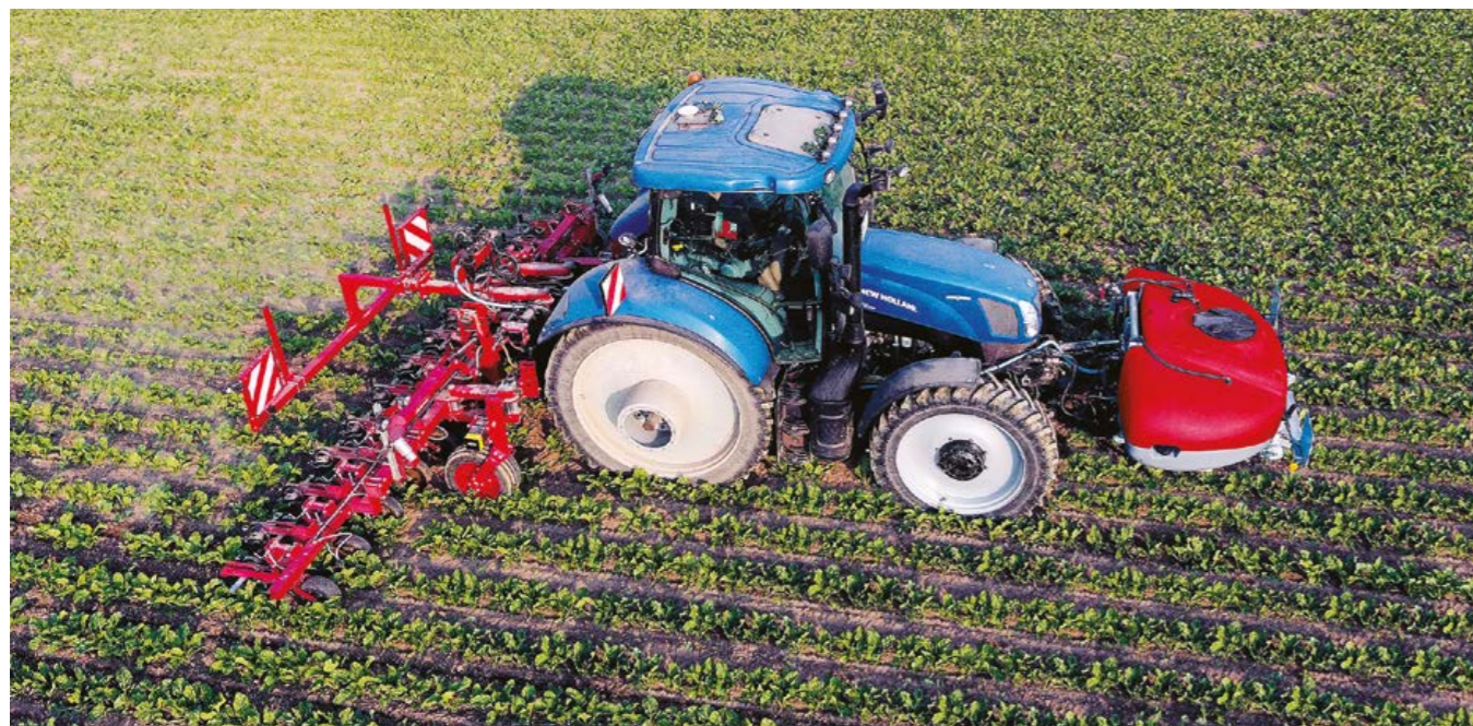
In-row spraying via the Steketee SprayKit applicator is possible via the SprayHub front tank connected to a rear-mounted inter-row hoe
