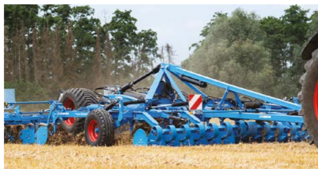
The new Karat 10 three-row cultivator has a more efficient design than its predecessor, with tines now arranged around the axis of greatest tension in work
