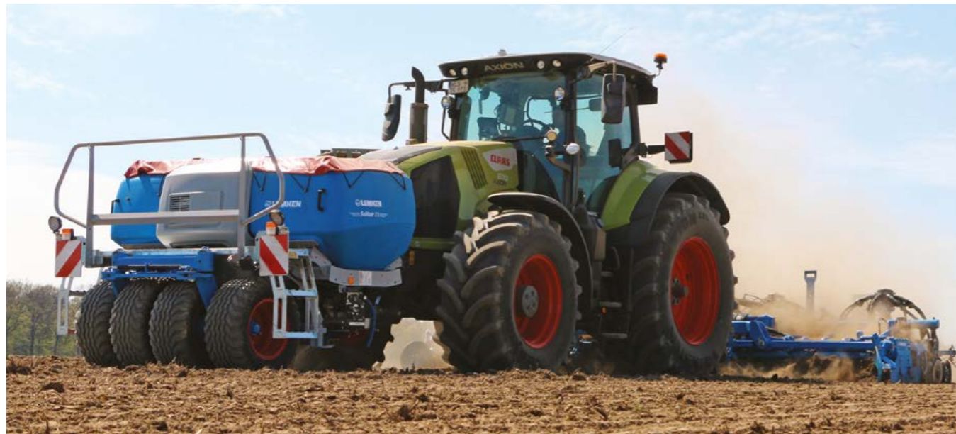
Lemken's Solitair 23+ front hopper and OptiDisc 25 coulters bar pairing is now ISOBUS-compatible
